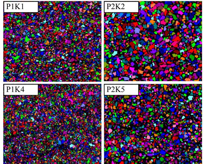
Figure 3: Clusters of carbides associated to objects through one of the 20 studied fields (X7000) for each coating
