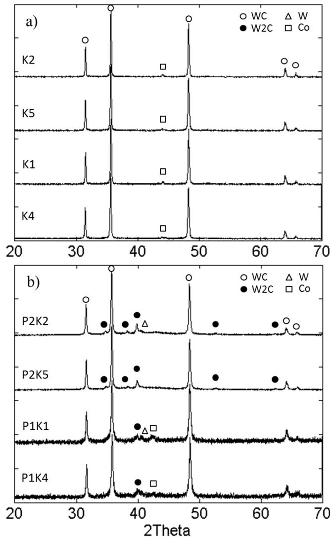
Figure 5: XRD patterns of powders (a) and coatings (b) with identification of principal phases
